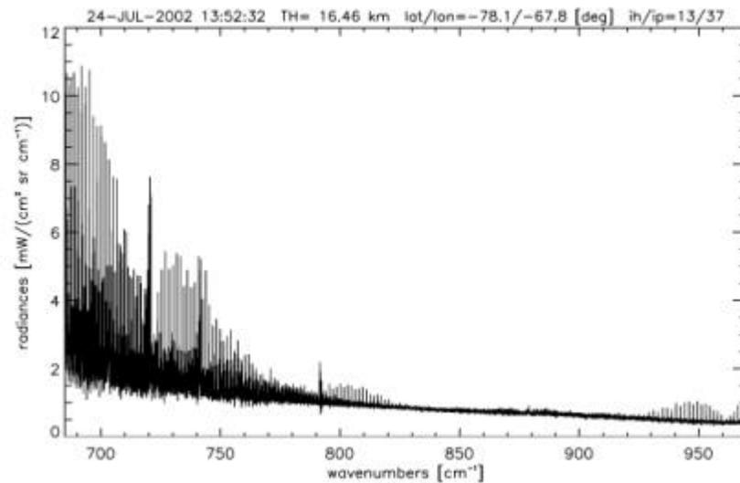
**Figure 9:** MIPAS band A spectrum in orbit 2082 of an optically thick polar stratospheric cloud at 16.5 km height. Radiance units in micro W/cm<sup>2</sup> sr cm<sup>-1</sup>.
