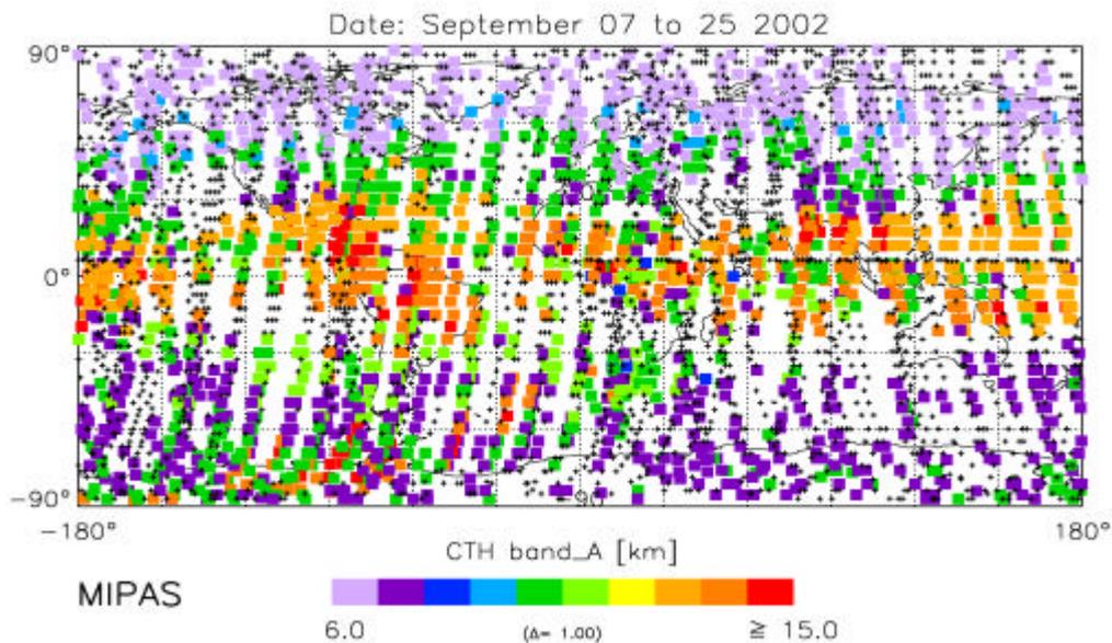
**Figure 11:** The first global cloud top height map computed from MIPAS level 1b data using CI-A with a threshold of 1.8. The appearance of cirrus clouds in the tropical upper troposphere and polar stratospheric clouds in the Antarctic polar winter can be observed.
