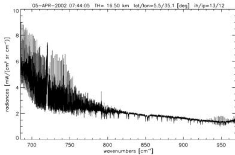
**Figure 8:** MIPAS spectrum of orbit 504 of an optically thick cirrus cloud including absorption features in the equatorial region (16.5 km tangent height). Radiance units in micro W/cm<sup>2</sup> sr cm<sup>-1</sup>.
