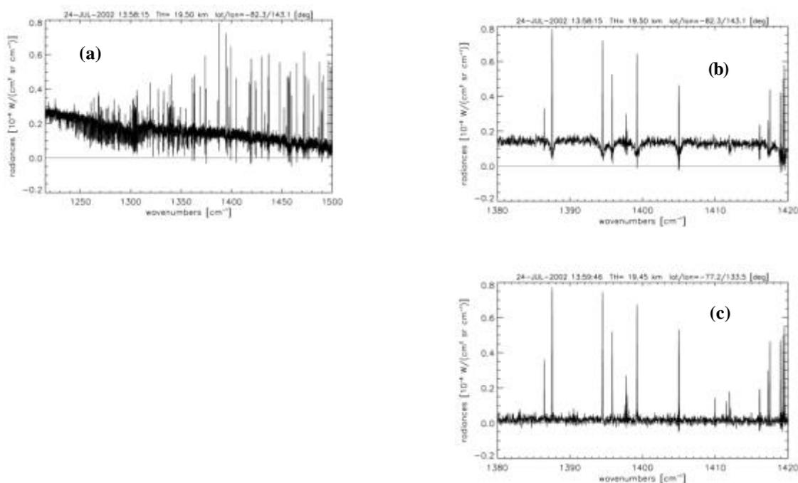
**Figure 10:** First spectrum of an Antarctic vortex PSC observed by the MIPAS on ENVISAT. Data are provided by the ESA and are preliminary but with expected calibration suitable for this purpose. (a) PSC at 19.5 km tangent height as observed in the MIPAS B band; (b) Detailed section of the same PSC spectrum near 1400 cm<sup>-1</sup>; (c) “Clear sky” spectrum at 19.45 km for a nearby profile. Radiances are in units of  $10^{-4} W/(cm^2 sr cm^{-1})$ .
