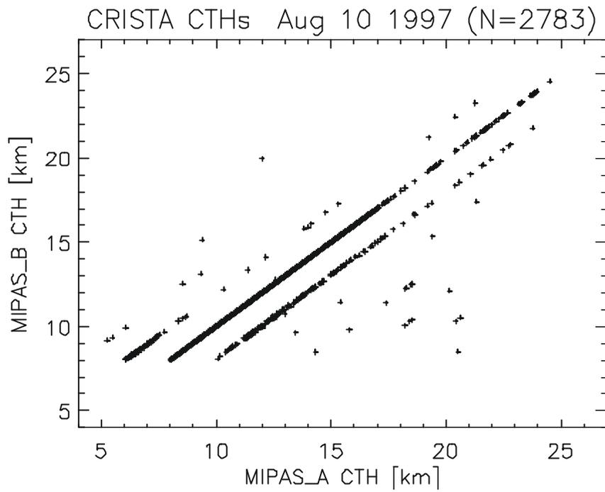
**Figure 5:** A comparison of cloud top height (CTH) computed from CRISTA data using the CI-A (MIPAS band A) and CI-B (MIPAS band B) indices. The data are for the left and right viewing directions of CRISTA on August 10<sup>th</sup> 1997.
