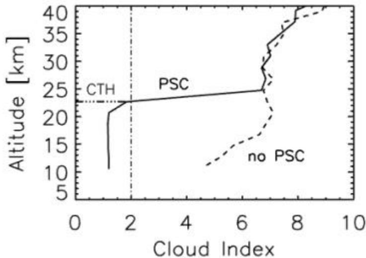
**Figure 2:** CRISTA cloud index profile [5] for clear sky and cloudy conditions (PSC). A threshold value of 2 - used for the CRISTA analyses - as well the cloud top height (CTH) are indicated by the dash-dotted lines.
