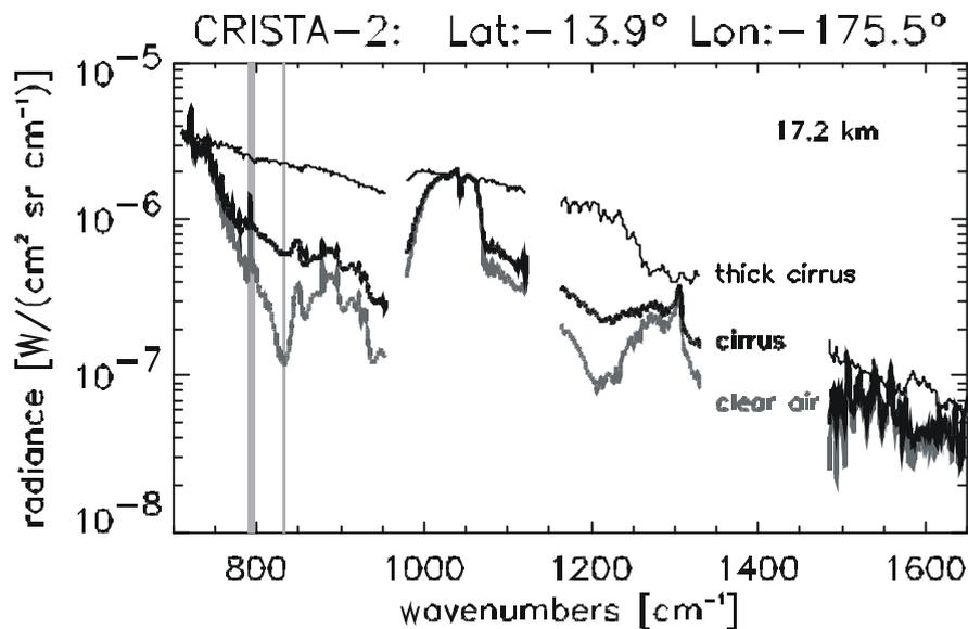
**Figure 1:** CRISTA spectra of optically thick and thin cirrus clouds as well cloud-free conditions in the tropical region at around  $17 \text{ km}$  tangent height measured in August 1997. The lines mark the locations of the CI-A mesowindow pairs.
