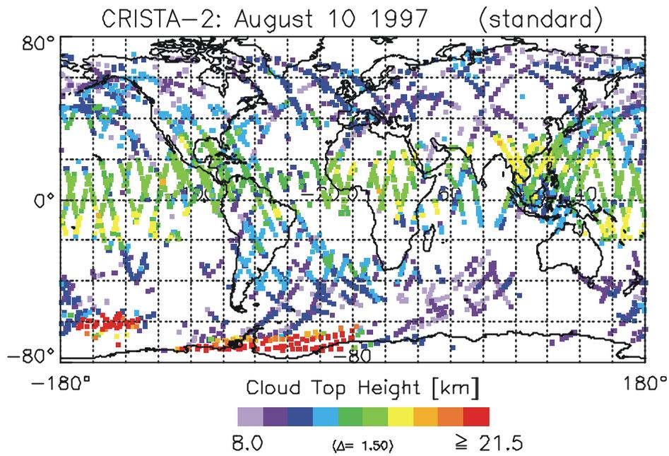
**Figure 3:** Cloud top height (CTH) computed from CRISTA data using the standard CRISTA index, CI-CR, which is the same as the MIPAS CI-A index. Only the left and right viewing directions of CRISTA were used because the detector of the central spectrometer for the wavelength region equivalent to MIPAS cloud index CI-B had problems in its calibration. Data are for August 10<sup>th</sup> 1997.
